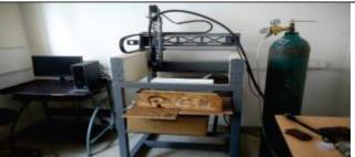
GMAW based Wire Arc Additive Manufacturing
