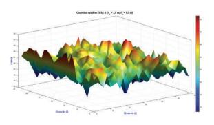
Fig. 5b Gaussian random field representing spatial distribution of internal friction angle of MSW
