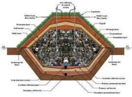
Fig. 5a Schematic representation of MSW landfill
