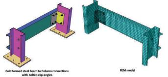
Fig.4 Cold formed steel connections between Beam- Beam & Beam-Column with clip angles under cyclic loading
